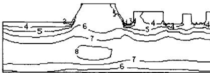
Fig. 3 Stress field of high pressure rotor of 300 MW steam turbine at rated load
