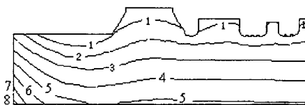
Fig. 4 Temperature field of high pressure rotor of 300 MW steam turbine at rated load
