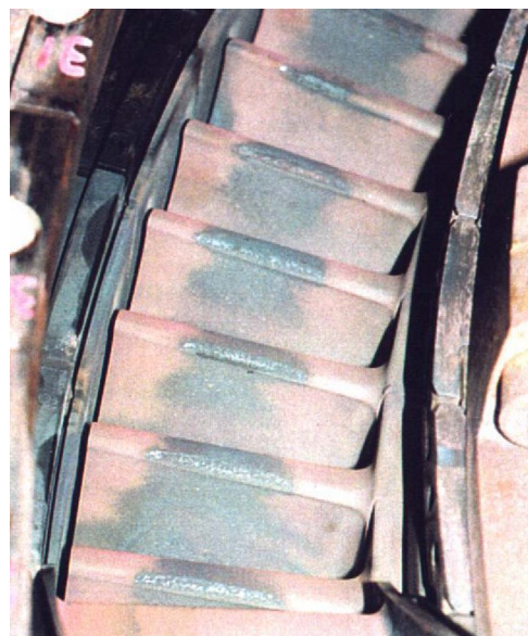
Fig. 10 Case history 3: cyclic oxidation damage on mounted first stage blades, leading edge side
